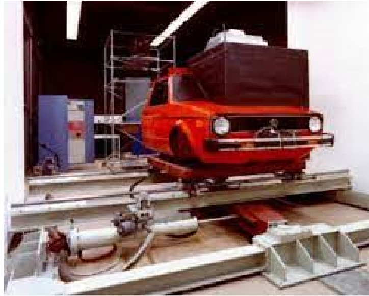
Figure 1.2 Driving simulator developed by Volkswagen [1]
