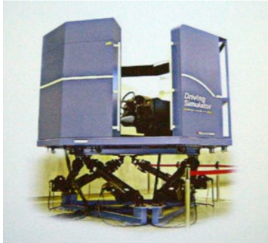
Figure 1.5 Driving simulator using a Stewart platform
