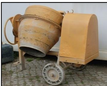
Fig.45 Betoneira 550 L - diesel
