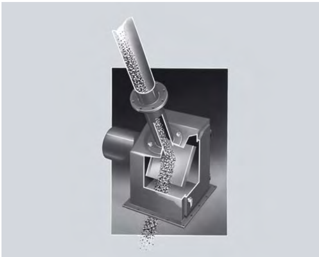
Solids flowmeter with sensing plate detail
