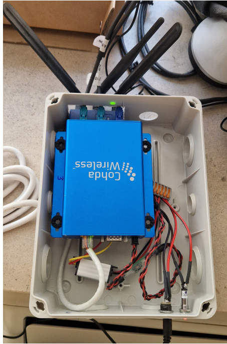
Figure 4.4: OBU Physical Setup
