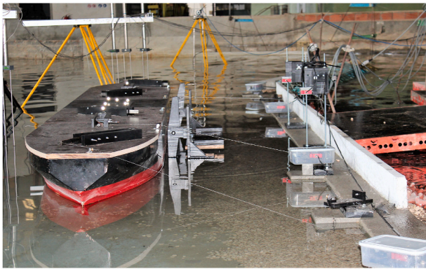
Fig. 7. Physical model of fenders and mooring lines.
