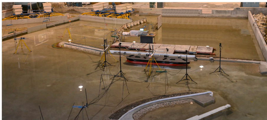
Fig. 3. The physical model of Leixões port at LNEC's wave basin.
