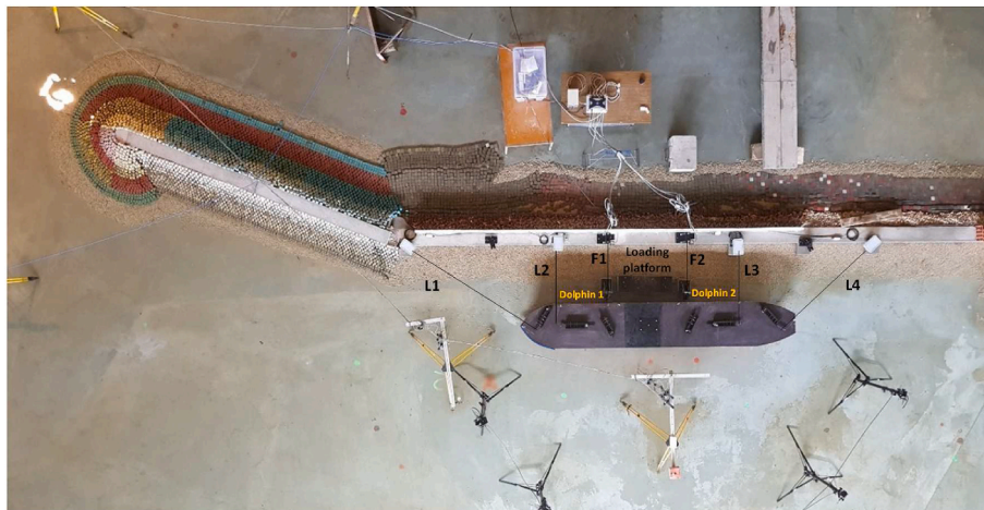
Fig. 6. The mooring arrangement in the physical model.
