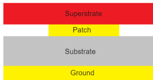
Figure 3.15: Structure of an antenna using superstrate.
