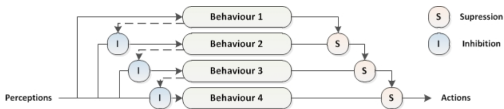
Figure 3 - Subsumption Architecture (adapted from Brooks, 1989)
