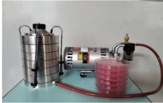
Figure 4: Andersen Six-Stages (Anderson Six Stage Bioaerosol Impactor Used for Air Sampling, n.d.).
