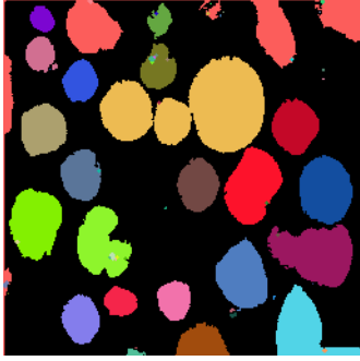
(a) Colored image of the segmentation of an etched micro-structure of titanium powder.
