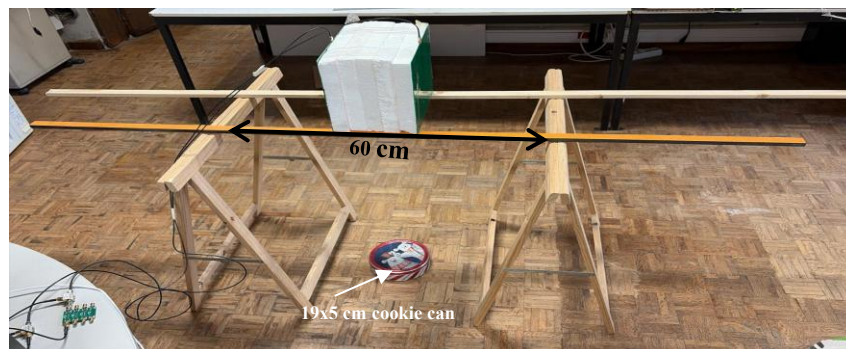
Figure 43- SAR experiment setup with antennas to the floor test with multiple targets without hardware cancelling
