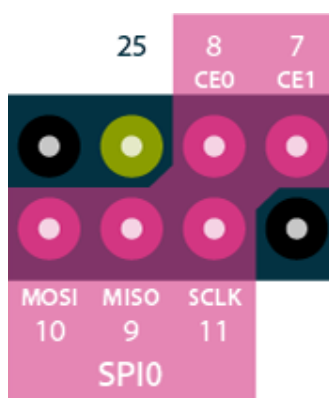
Figura 77. Pinout do Raspberry Pi (SPI) [36]
