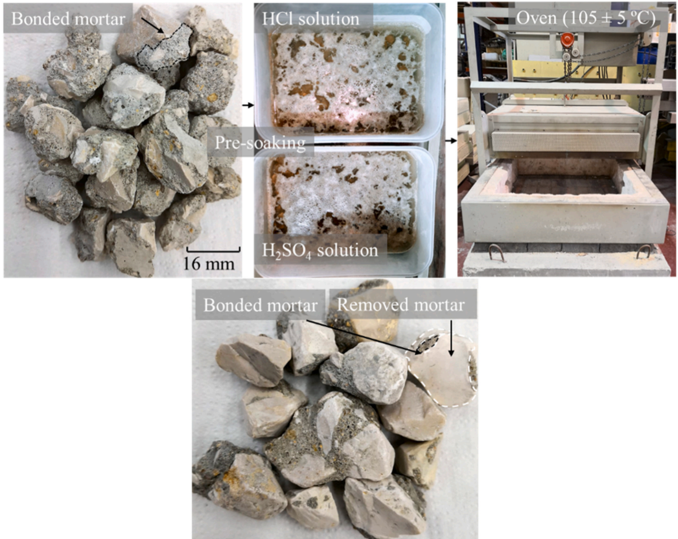
Fig. 2. - Pre-soaking treatment procedures for RCA.
