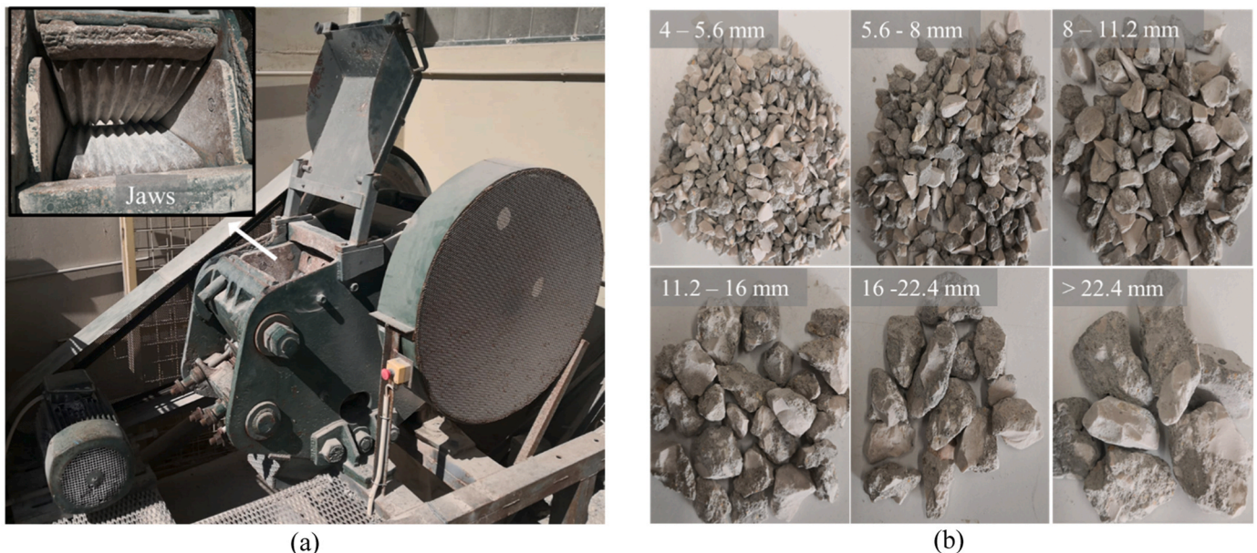
Fig. 1. - Jaw crusher used in the production of RCA (a); size fractions of RCA used in this study (b).
