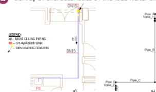
Figure 1. Section of Building C, Floor -2 from ISEL water distribution system in: a) AutoCad and b) EPANET 2.2.
