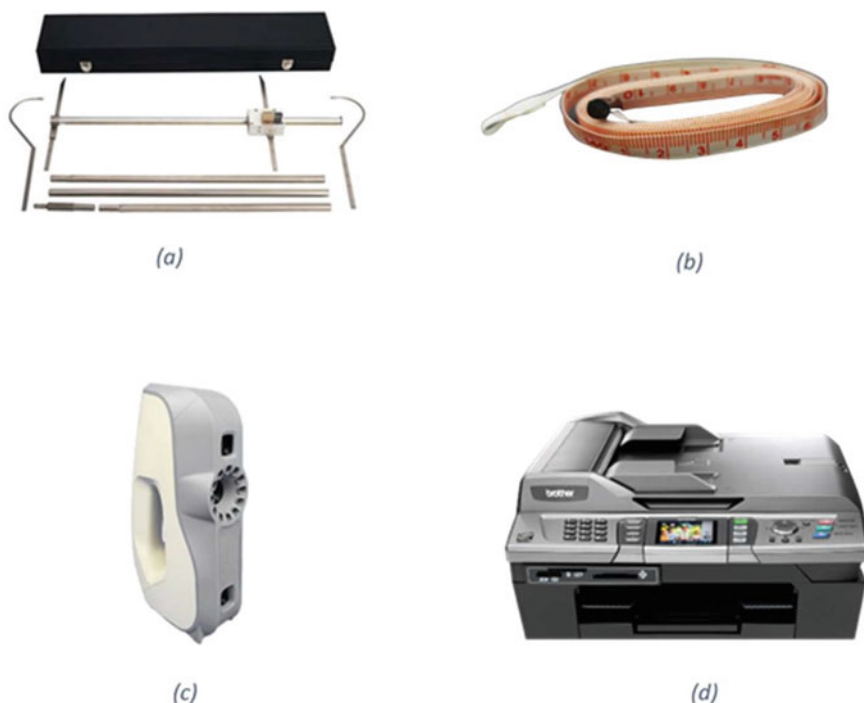
Fig. 2 Equipment used to measure participants' hand dimensions: a anthropometer; b measuring tape; c 3D scanner and d 2D scanner
