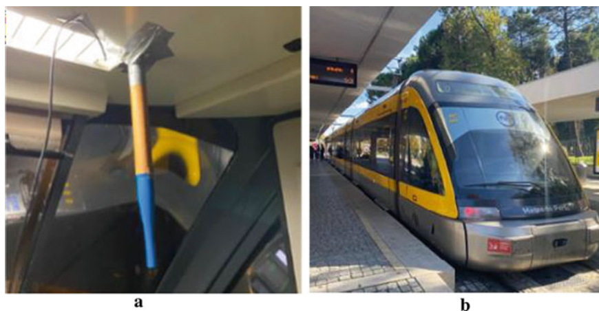
Fig. 1 a Blue microphone of the SAM Scribe system, suspended from the ceiling of the subway-driver's compartment, before attachment of wind shield. b Eurotram—model of the vehicle in which recordings were performed
