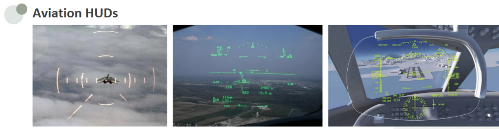
Figure 2.2: Pictured are several examples of the use of HUDs in aviation: on the left, a U.S. Navy jet can be seen aligned in the HUD of another aircraft; the two images on the right show how flight-related data can be displayed to aid the pilot.
