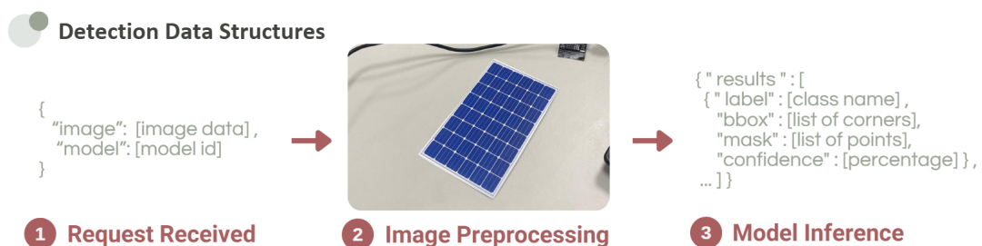
Figure 5.3: Main data structures from the first three steps: 1) Request format; 2) Image frame; 3) Detection result format.
