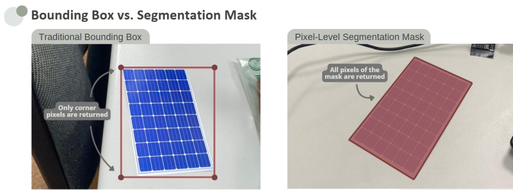
Figure 5.1: Examples of YOLO detection formats: on the left, a bounding box is constructed from the detected corners; on the right, a pixel-level mask captures all detected points.
