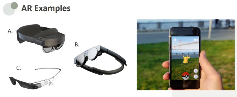
Figure 2.4: Some AR technologies can be seen: A. Holo Lens Pro 2 , B. Magic Leap 2 and C. Google Glass Enterprise Edition 2 . To the right, a smartphone-based application ( Pokémon Go ) is also shown: this technology overlays virtual objects atop real environments.
