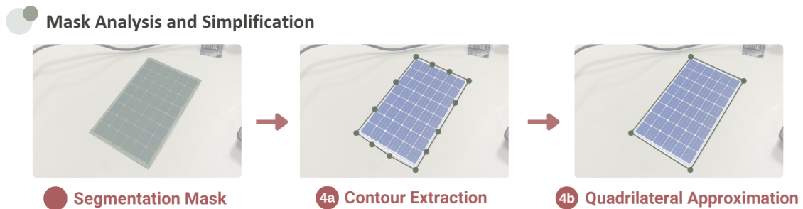
Figure 5.4: Reference for the mask analysis steps: The segmentation mask (left) identifies every pixel that belongs to the detected object. Step 4a extracts only the outer contour, reducing the pixel amount. In step 4b, the contour is further approximated into a quadrilateral, keeping only the four most relevant corner points.
