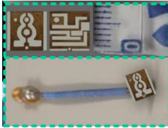
Figure 2.4: Bear shaped microstrip antenna for the 915 MHz ISM frequency band (taken from [15])
