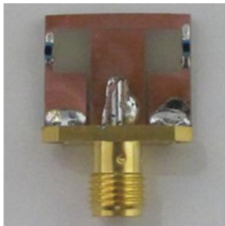
Figure 2.5: Compact zeroth-order resonance antenna operating in the MICS frequency band (taken from [17])
