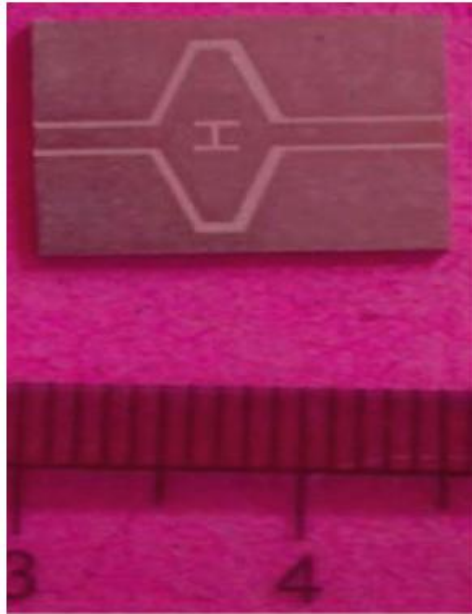
Figure 2.1: Implantable CPW fed monopole for 2.45 GHz ISM band (taken from [12])
