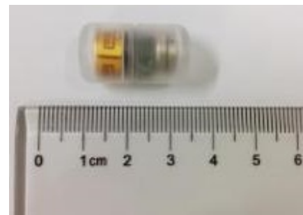
(b) Conformal antenna wrapped around capsule
