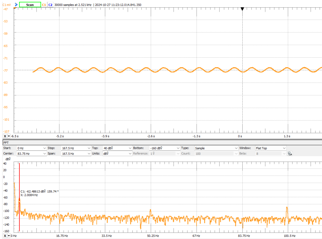
Figure 4.1: Sinusoidal signal in oscilloscope, f = 2 Hz, Real-Time (top subfigure) and FFT (bottom subfigure)
