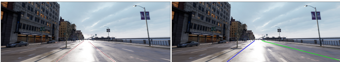
Figure 4: Ground truth (left) and lane detection (right). Glare from direct sunlight creates the most severe challenges.
