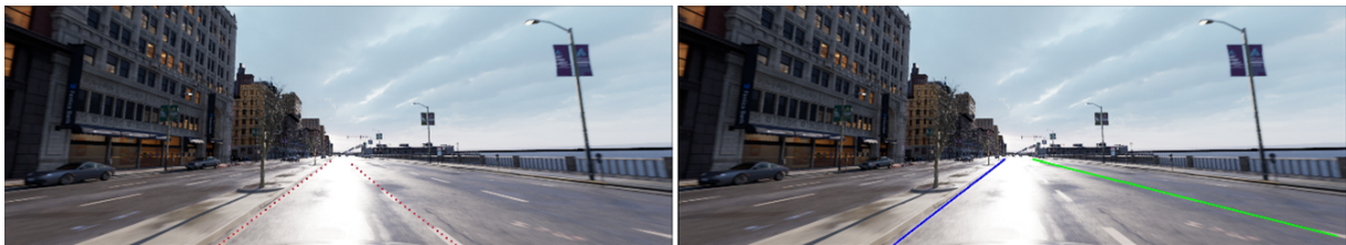
Figure 4.4 Glare from direct sunlight creates the most severe challenges.
