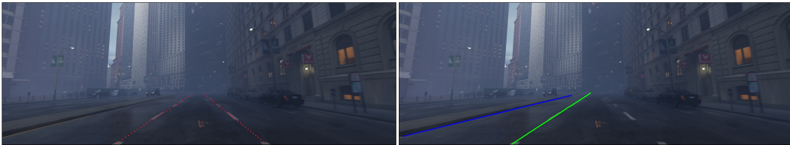
Figure 3: Ground truth (left) and lane detection (right). The model misinterpreted numerous frames in fog-filled scenes.
