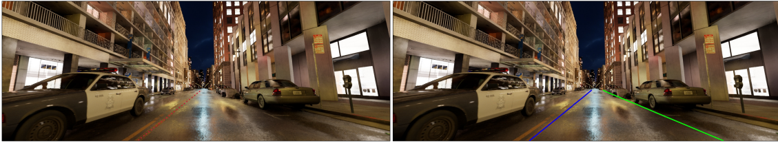
Figure 2: Ground truth (left) and lane detection (right). The model often inferred lane markings from parking boundaries.
