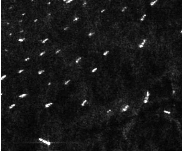
Figure 1.1 SAR image of vessels at sea represented by the white speckles
