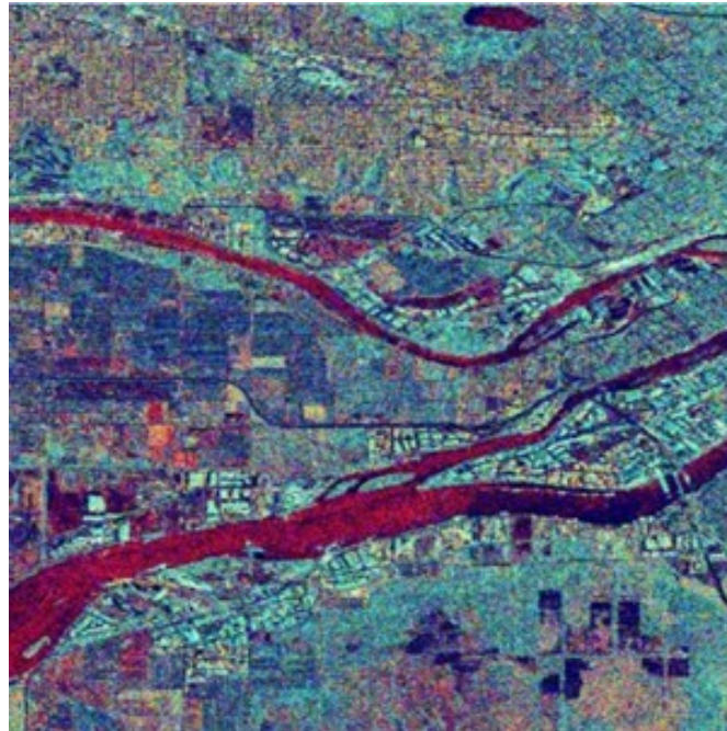
Figure 3.2 The RGB image obtained using the HH, HV, and VV polarizations
