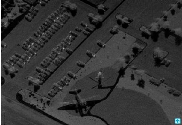
Figure 1.2 SAR image of a military hanger with the aircrafts and its shadows
