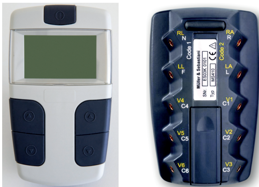
Figure 3.3 The left and right images show the front and back views of the MS410 device, respectively. The missing pushbutton contacts, visible in the right image, are inserted before starting the device, connecting and arranging the electrodes, and testing the acquisition device [27].
