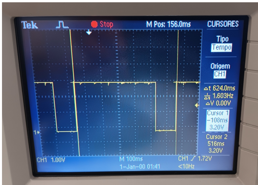
Figure 5.6 Producer task execution time, acquired using GPIO33, with an execution time of 624 ms. Sampling frequency: 800 Hz. BatchSize : 500 values. Note: Due to the duration of the task, the time window could not be expanded, possibly preventing a more precise measurement. Time scale: 100 ms.
