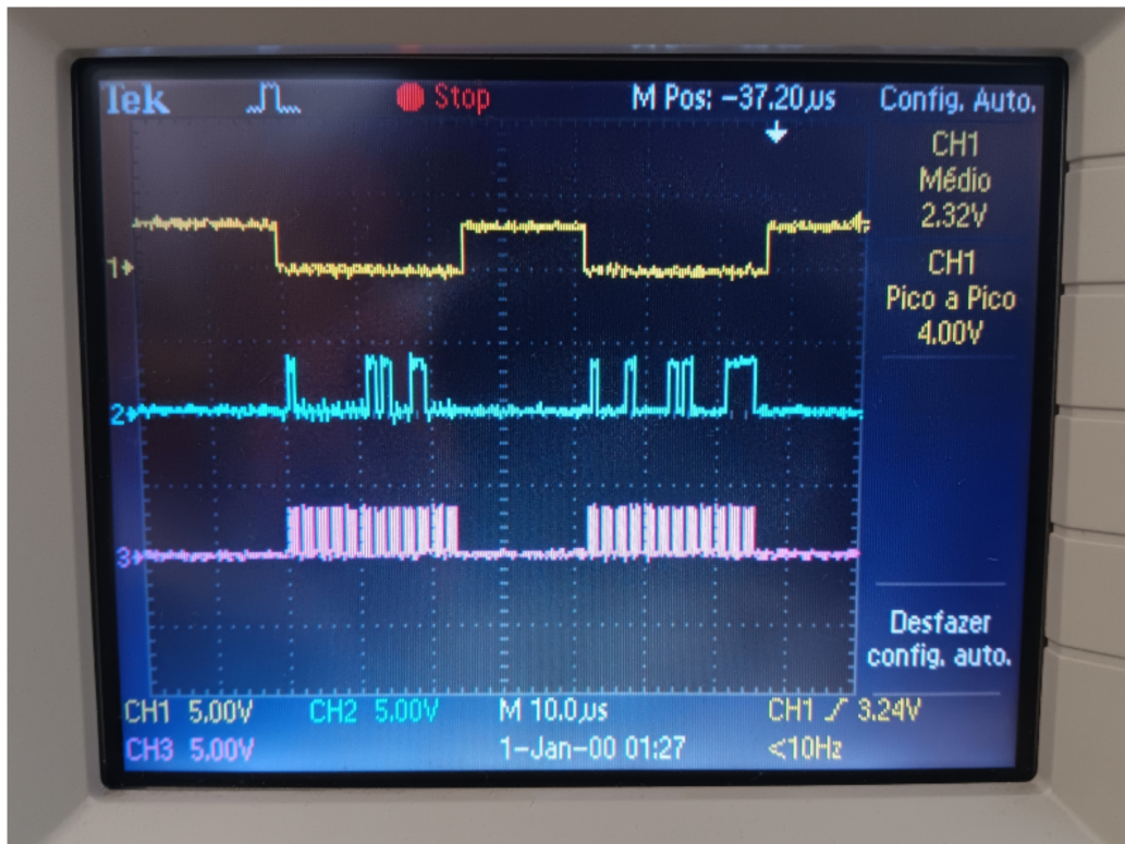
Figure 4.23 Data transmission between MCU and both MCP23S08 I/O expanders. Timescale 10\mu s . The yellow signal represents the \overline{CS} of both components. The blue signal corresponds to MOSI line. The purple signal corresponds to SCLK line.
