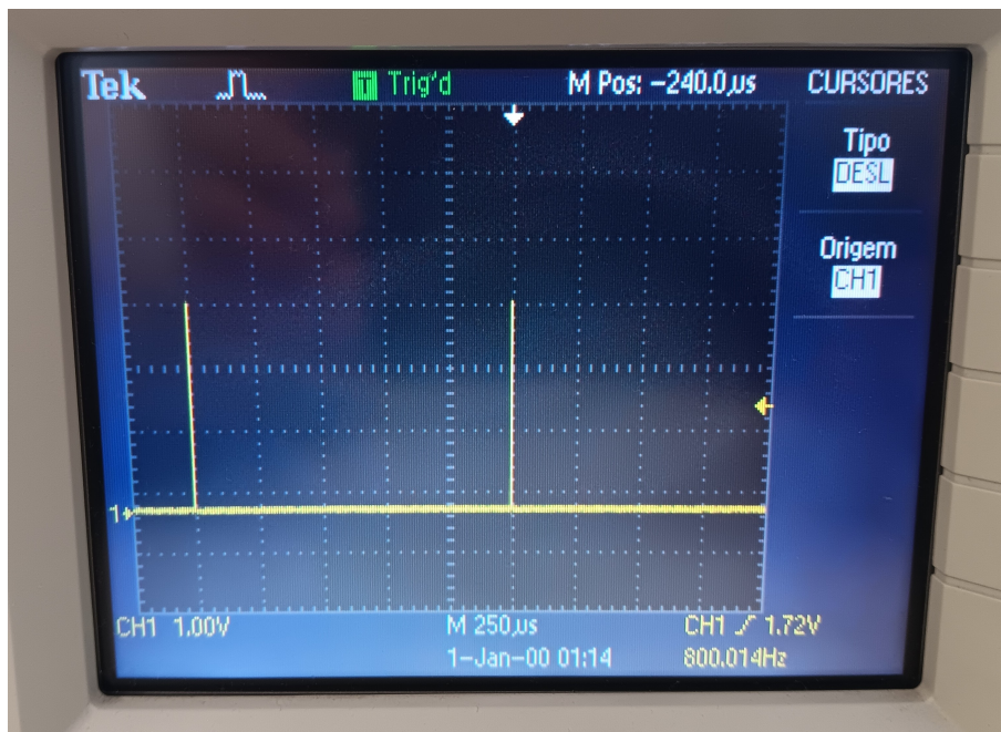
Figure 5.7 Interrupt routine execution time, acquired using GPIO32, with an execution time of 1.25 ms, correspondent to a sampling frequency of 800 Hz. Time scale: 250 \mu s .
