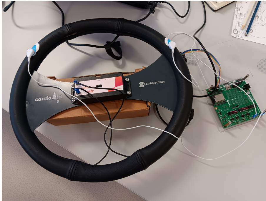
Figure 5.11 Experimental setup comprised of the ECG simulation system, Cardioleather acquisition device and two semi-dry electrodes. To prevent possible noise sources, the acquisition device was positioned on top of a box.
