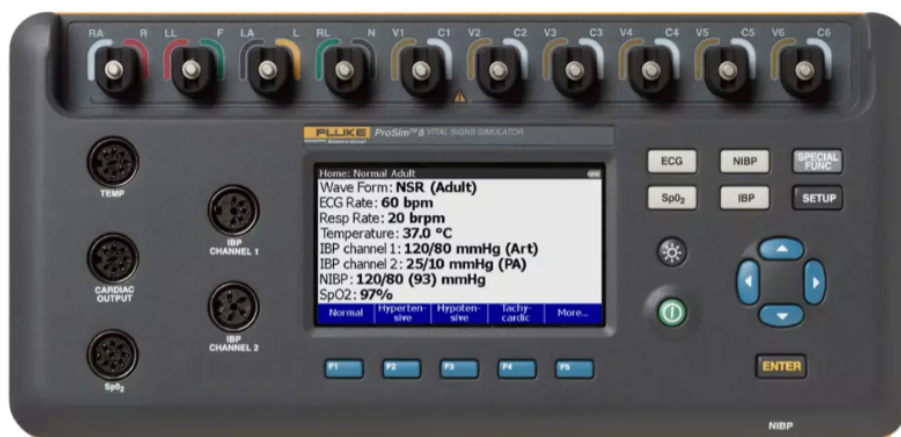
Figure 3.1 Top view of Fluke Biomedical ProSim8 patient simulator. On the left side, the device features 5 connections associated with invasive blood pressure, temperature, oxygen saturation and cardiac output. The top side presents 10 connectors for ECG waveforms simulation labeled, respectively, according with AHA and International Electrotechnical Commission (IEC) in the left and right sides. The center and right sides presents user interface capabilities [25].
