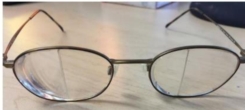
Figure 4. Hemi-prism ground in to spectacles. This is ground in base right whereas the patient's prism would be ground in base left.
