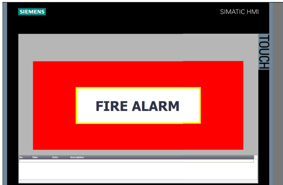
Figure 4.8: Fire Alarm screen.
