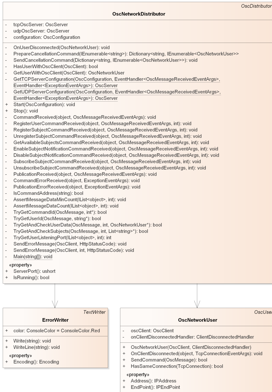
Figure C.2: Structure of the OSC Network Distributor
