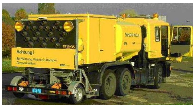
Figura 3.19 – Stuttgarter Reibungsmesser [TYROSAFE, 2008]
