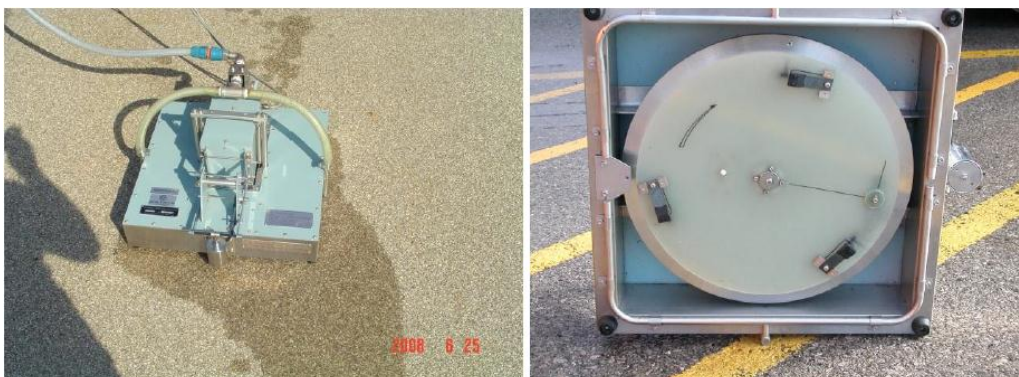
Figura 3.3 – Dynamic Friction Tester [Rodriguez, 2009]
