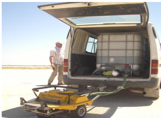
Figura 4.4 – GripTester do LNEC
