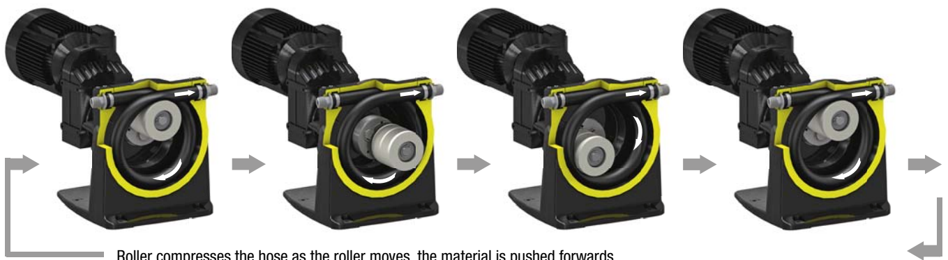
Roller compresses the hose as the roller moves, the material is pushed forwards.
