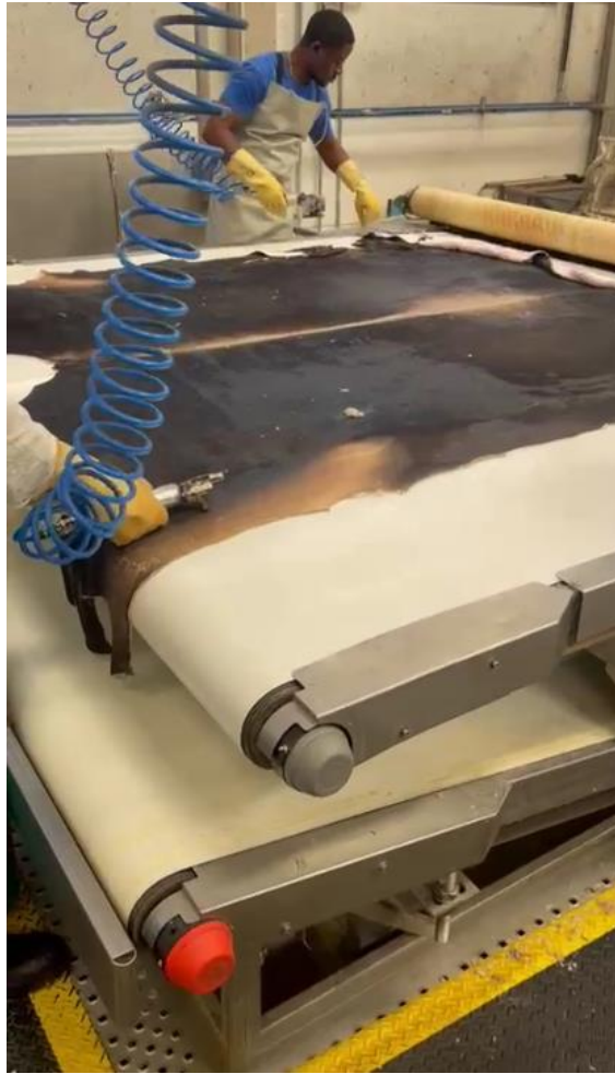
Figure 4.16 - Belt conveyor and cutting line.
