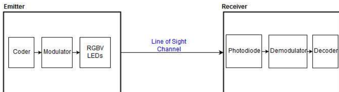
Figure 3-1: Block diagram of the VLC system for illumination, positioning and data transmission
