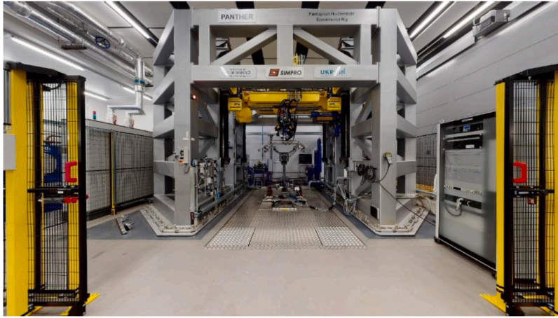
Fig. 5. Panther, full-scale pantograph test facility.
