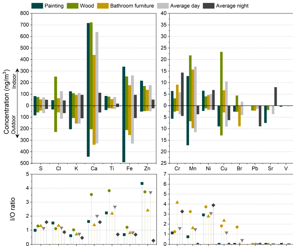
Fig. 5. Top: Concentrations of PM 10 -bound elements in different store sections and mean value for the day and night periods. Bottom: Indoor / Outdoor ratio.
