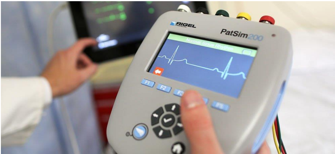
Figure 36: Front view of the RIGEL medical PatSim200, in this picture the device appears to be testing an ECG monitor, generating a normal ECG waveform [89]
