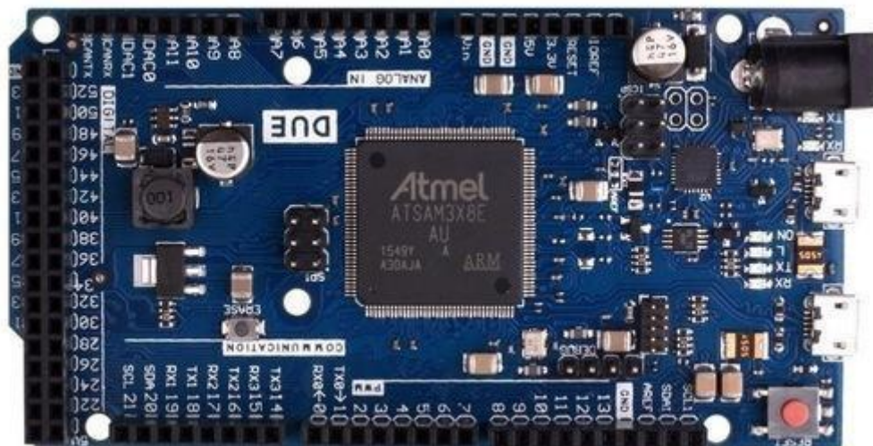
Figure 2.2.2. Arduino Due board (top view) [22]
