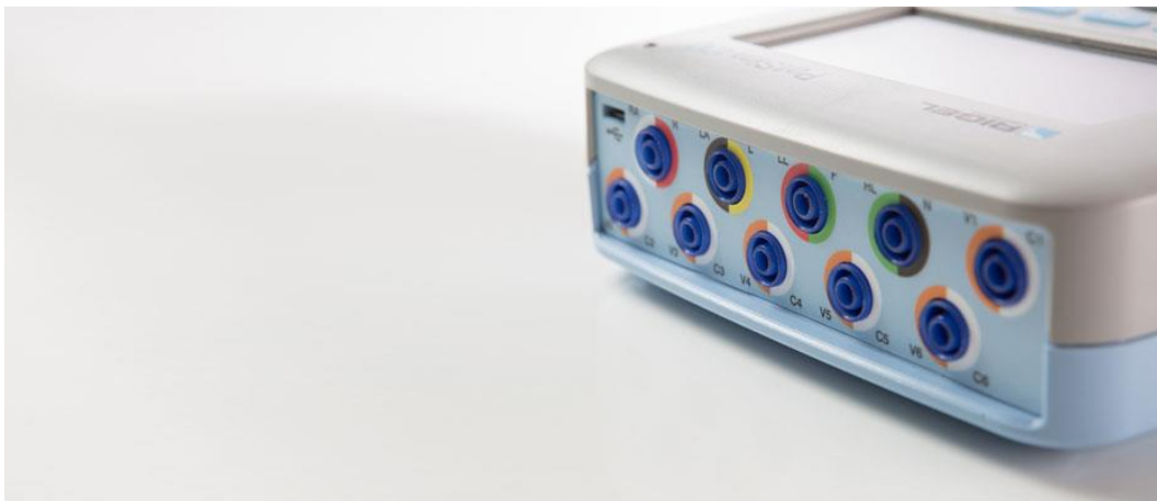
Figure 35: Side view of the RIGEL PatSim200, showing the ECG output jacks[88]
