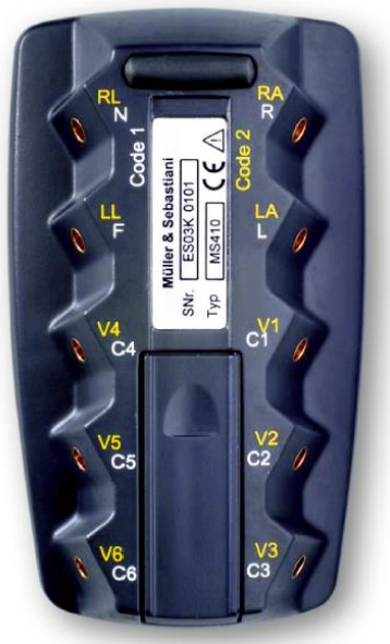
Figure 38: Back view of the MedTec MS410, showing the signal output jacks [91]
