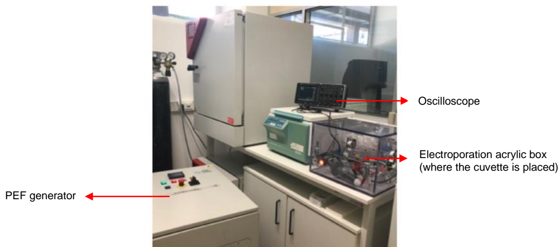
Figure 4.6. EPULSUS-LPM 1B-10 equipment inside culture room for PEF applications.
