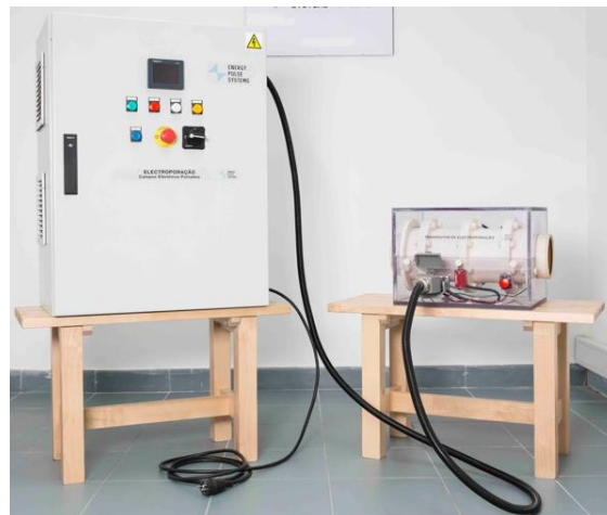
Figure 1.6. Example of Industrial PEF equipment from the Portuguese company Energy Pulse Systems .
