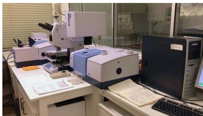
Figure 4.10. FTIR equipment: VERTEX 70 spectrometer from Bruker equipped with an HTS-XT module, also from Bruker, connected to a computer for data acquisition obtained by OPUS software, from Bruker.
