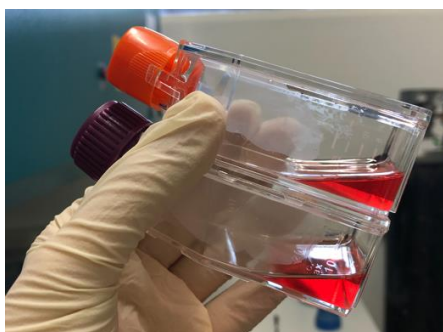
Figure 4.5. Two different T25-Flasks (25cm 2 of adhesion surface) with Nunclon Delta treated surface for cell culture.
