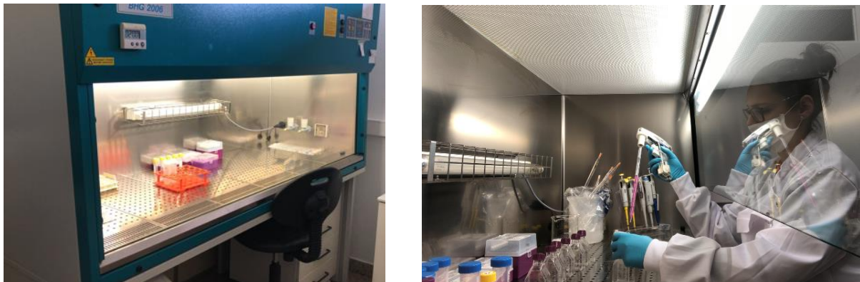
Figure 4.2. Left: Laminar vertical flow cabinet. Right: Work inside the laminar flow cabinet, using the automatic motorized pipette to remove culture medium.
