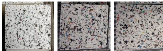
Figure 3. Plastic Residue addition to plaster mix in 50%, 60% and 70%
