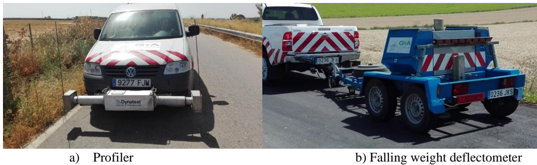
Figure 2. Images of the FWD and Profiler a) and FWD b) in the Experimental Section
