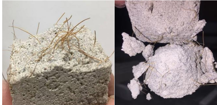
Figure 1. Mortars with coconut fiber specimens after failure.
