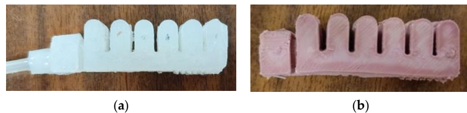
Figure 3. PneuNet actuators of type 1 fabricated with molds (a) made with DragonSkin Fast 10 silicone and (b) made with Elastosil M4601 A/B silicone.
