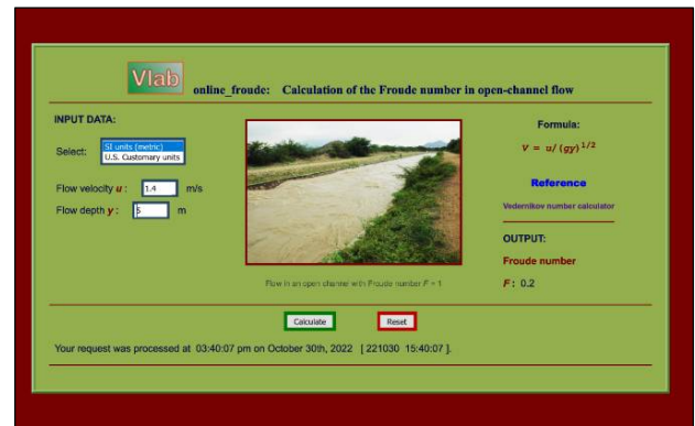
Figure 2 Ponce’s Problem No. 143 A (in Hydraulics): Calculation of the Froude number in open-channel flow.
