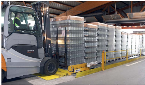
(a) Sistema de conveyors.
