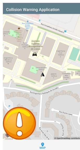
Figure 4.5: Collision warning application detecting a possible collision.
