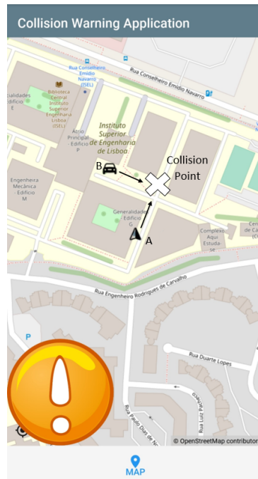
Figure 4.6: Collision warning application detecting a collision (visual assist).
