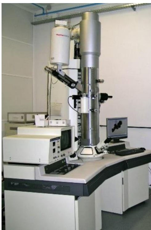
Figura 26 - Analytical TEM: Hitachi 8100 com ThermoNoran light elements EDS detector and digital image acquisition.
