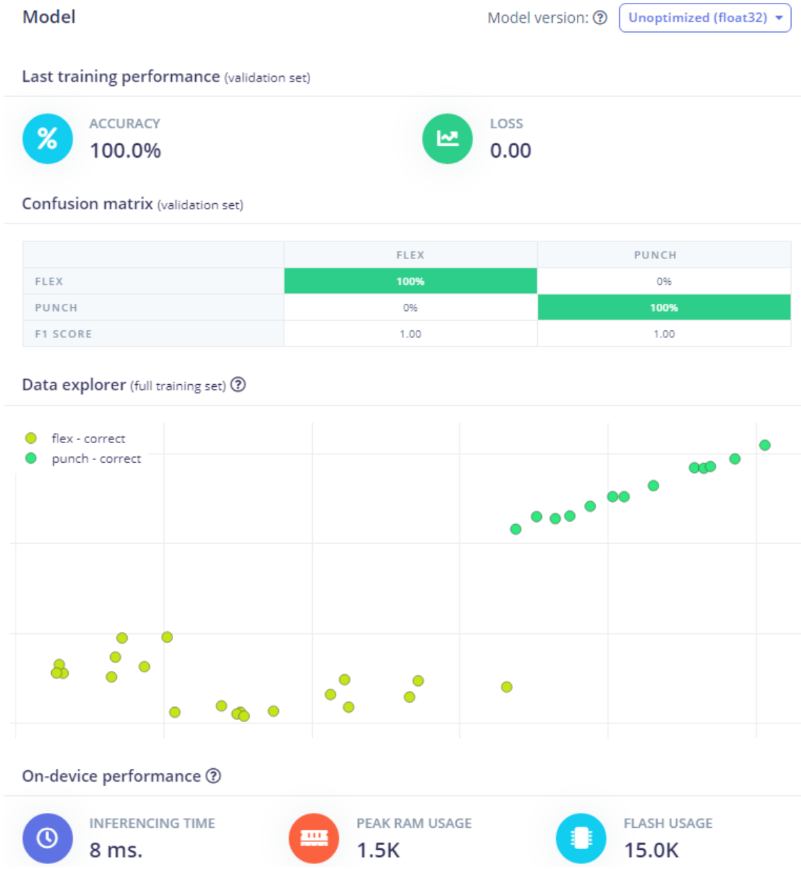
Figure 3.13: IMU classifier with TensorFlow Lite using Edge Impulse: Model from Edge Impulse Platform.
