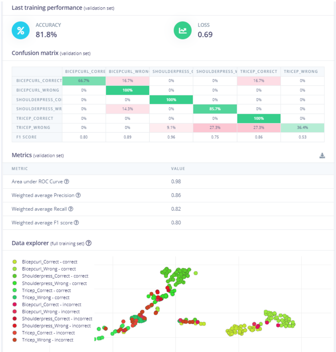
Figure 9.2: Edge Impulse training performance including all the six exercises using as a processing block spectral analysis.
