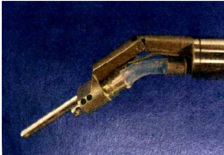
Fig. 35 - Prototype laparoscopic laser delivery device [138].
