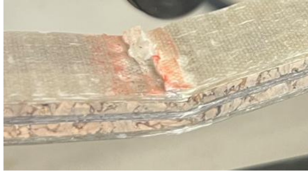
Figure 2.27 – T3 Specimen Face Wrinkling
