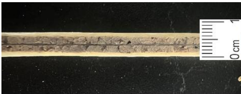
Figure 3.3 - T2 (4F/1C/2F/1C/4F) Sandwich Specimen.
