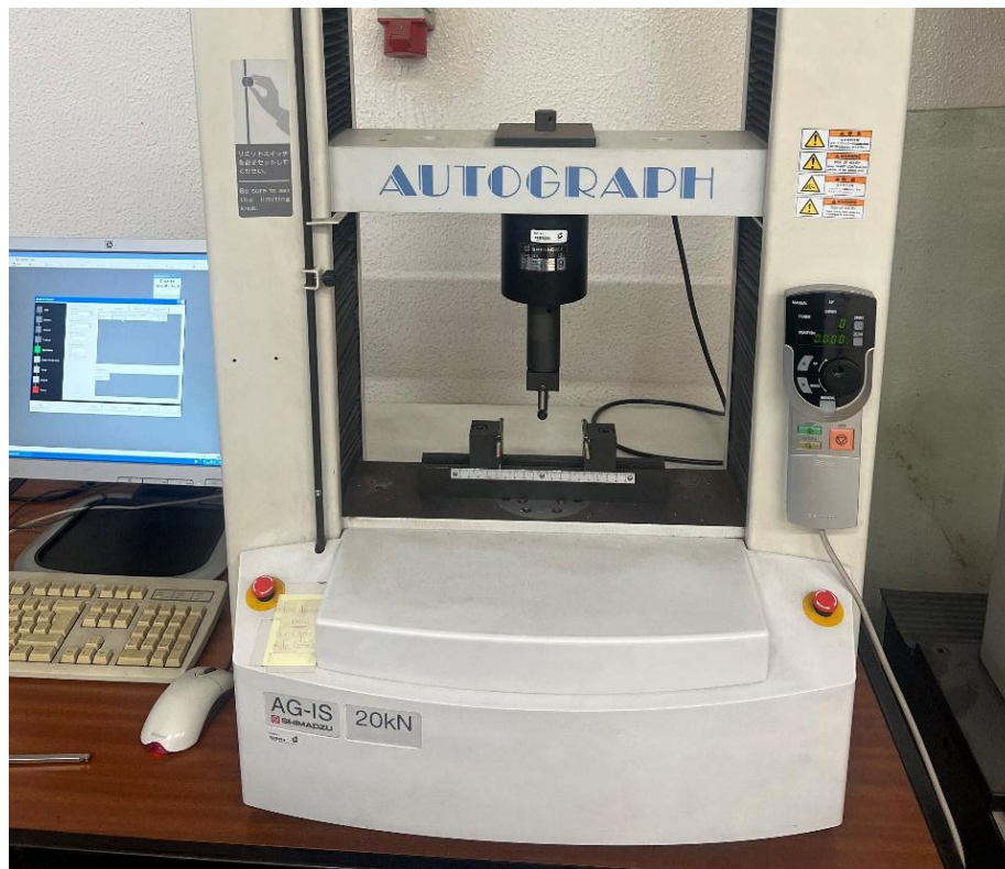
Figure 3.7 – Universal testing machine with 3 point bending test fixture mounted.
