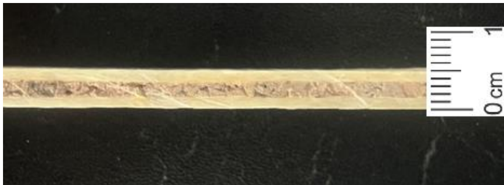
Figure 3.2 - T1 (5F/1C/5F) Sandwich Specimen.
