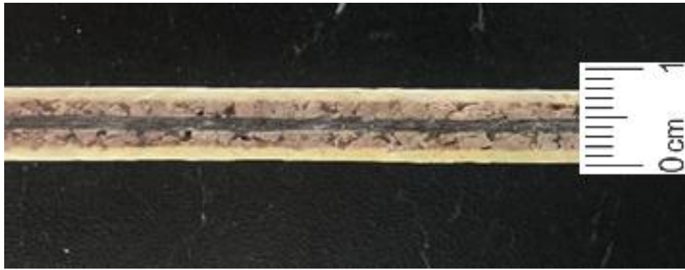
Figure 3.4 - T3 (5F/1C/5F/1C/5F) Sandwich Specimen.
