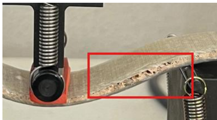
Figure 5.1 - T1 specimen core crack.
