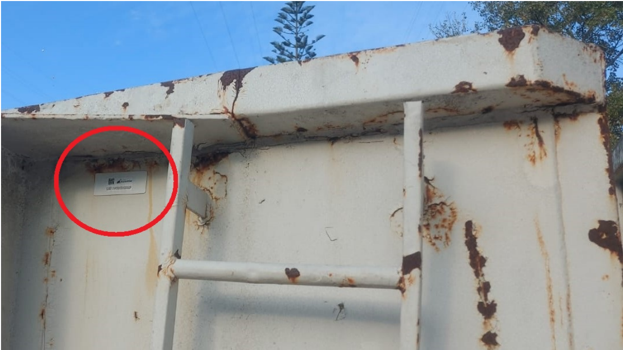
Figure 5.13: Container with tags (printed passive RFID tag)
