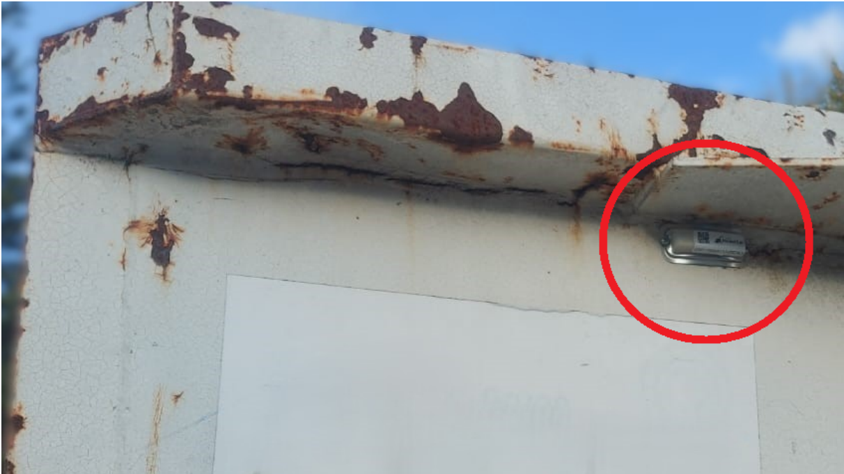
Figure 5.12: Container with tags (rigid passive RFID tag)
