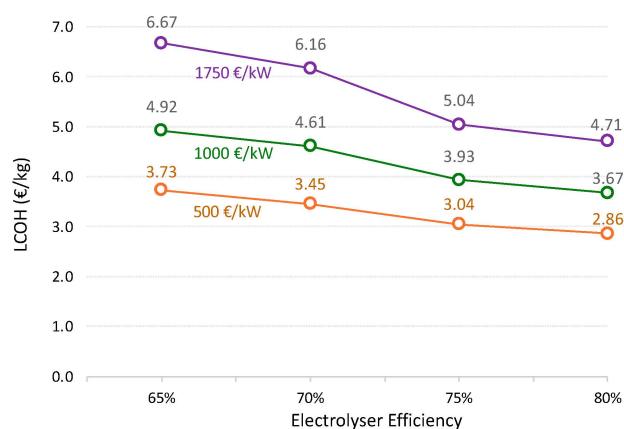
Figure 8. LCOH as a function of the electrolyser efficiency for three levels of Capex: 500 EUR/kW, 1000 EUR/Kw, and 1750 EUR/kW (EUR/kg).
