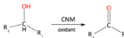
Scheme 1: Oxidation of alcohols to aldehydes or ketones catalysed by C-dots prepared from cork industry wastewater.
