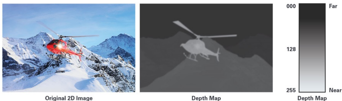
Figure 2.3 Example of a ToF depth map. Extracted from [30].
