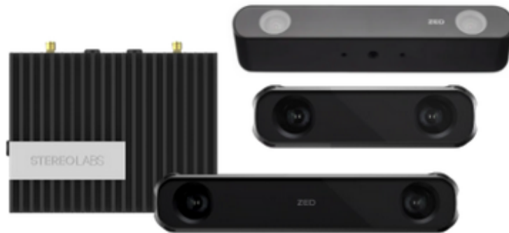
Figure 1.1: Stereoscopic ZED series cameras and ZED Box with a NVIDIA Jetson board.
