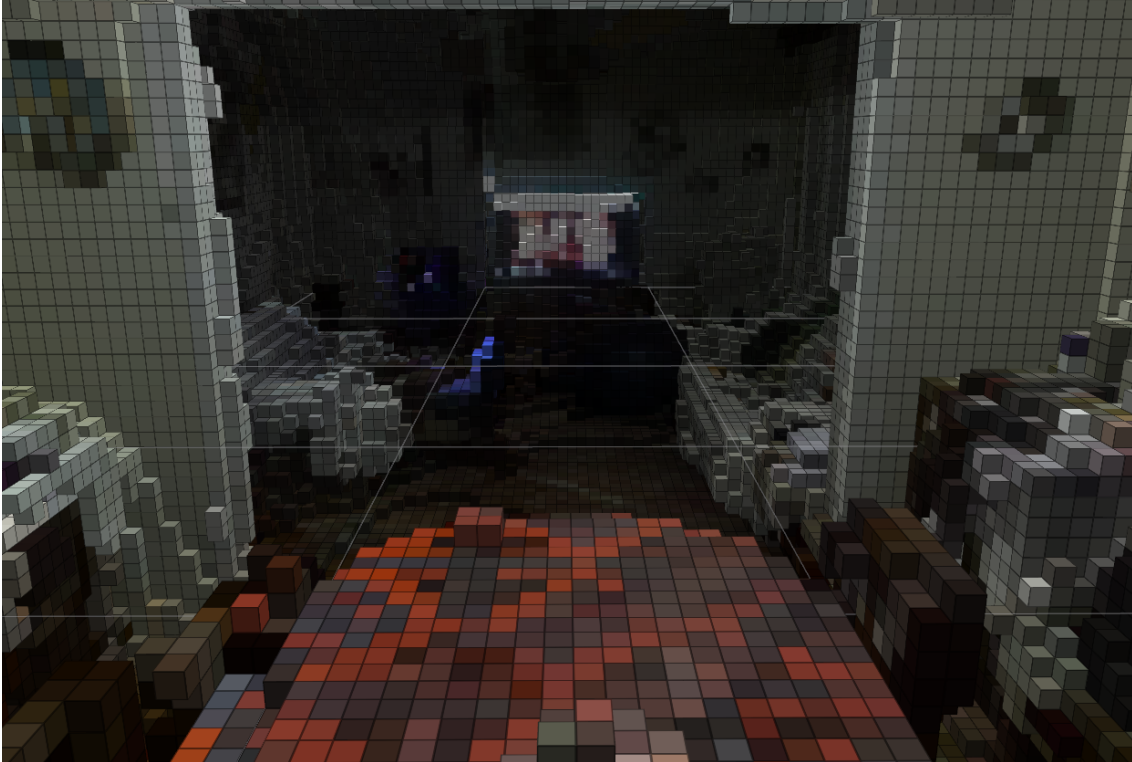
Figure 3.12: OctoMap of a living room, represented using boxes in RViz2.
