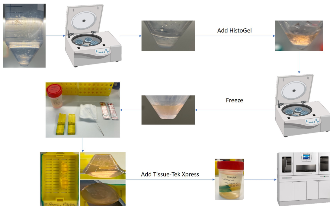
Figure 3.5: Overview of the histology protocol. The organoids were centrifuged and the supernatant was removed. The heated histogel was added to the pellet. This mixture was centrifuged and frozen at -20^{\circ}\text{C} for five minutes. Using a scalpel, the gel was sliced and placed in a cassette. The cassette was placed in Tissue-Tek Xpress x120.
