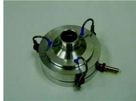
Impactation mechanism and active sampling device (Andersen one stage)
