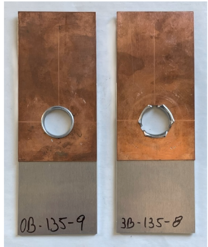
Fig. 6. Side-by-side joints without and with branches.
