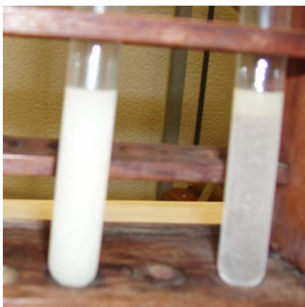
Figure 18 - W/O and O/W emulsions using SFAE from sucrose and rapeseed FAME, with a DE of 3.
