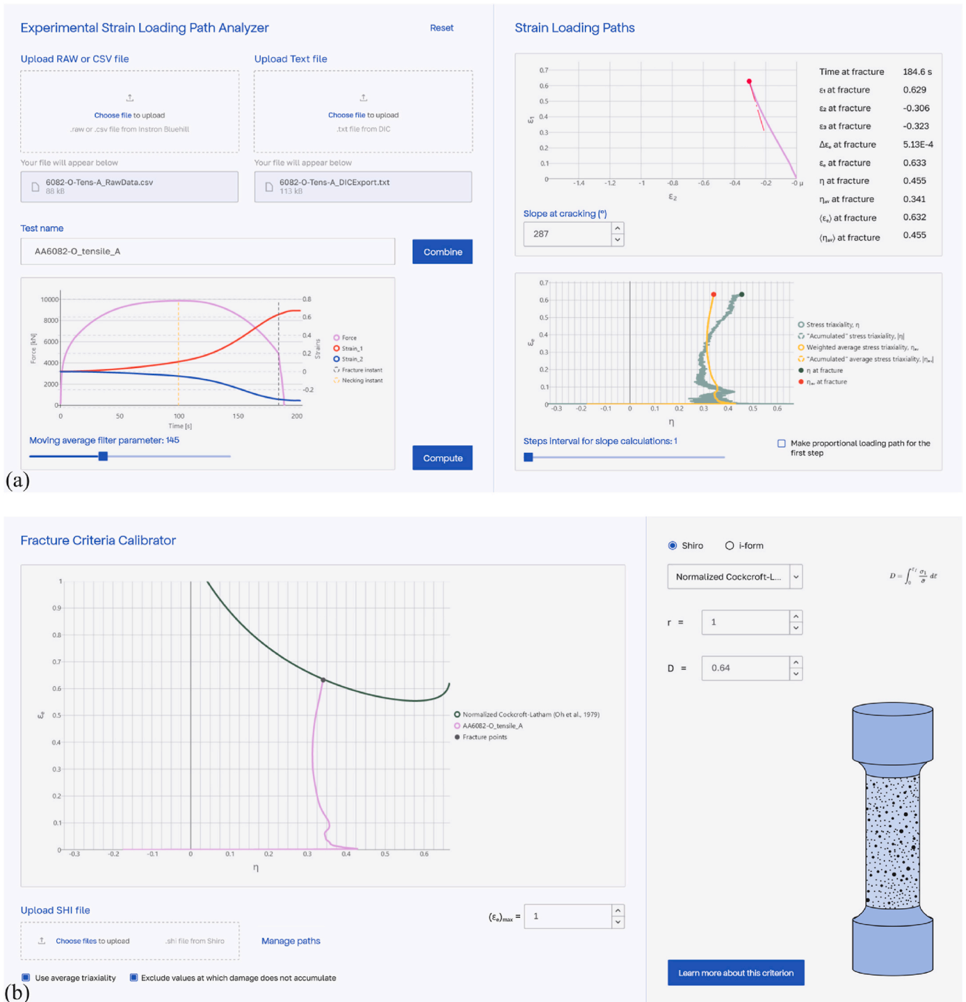
Fig. 6. Screenshots of the (a) analyzer and (b) calibrator user interfaces for a rod tension test.
